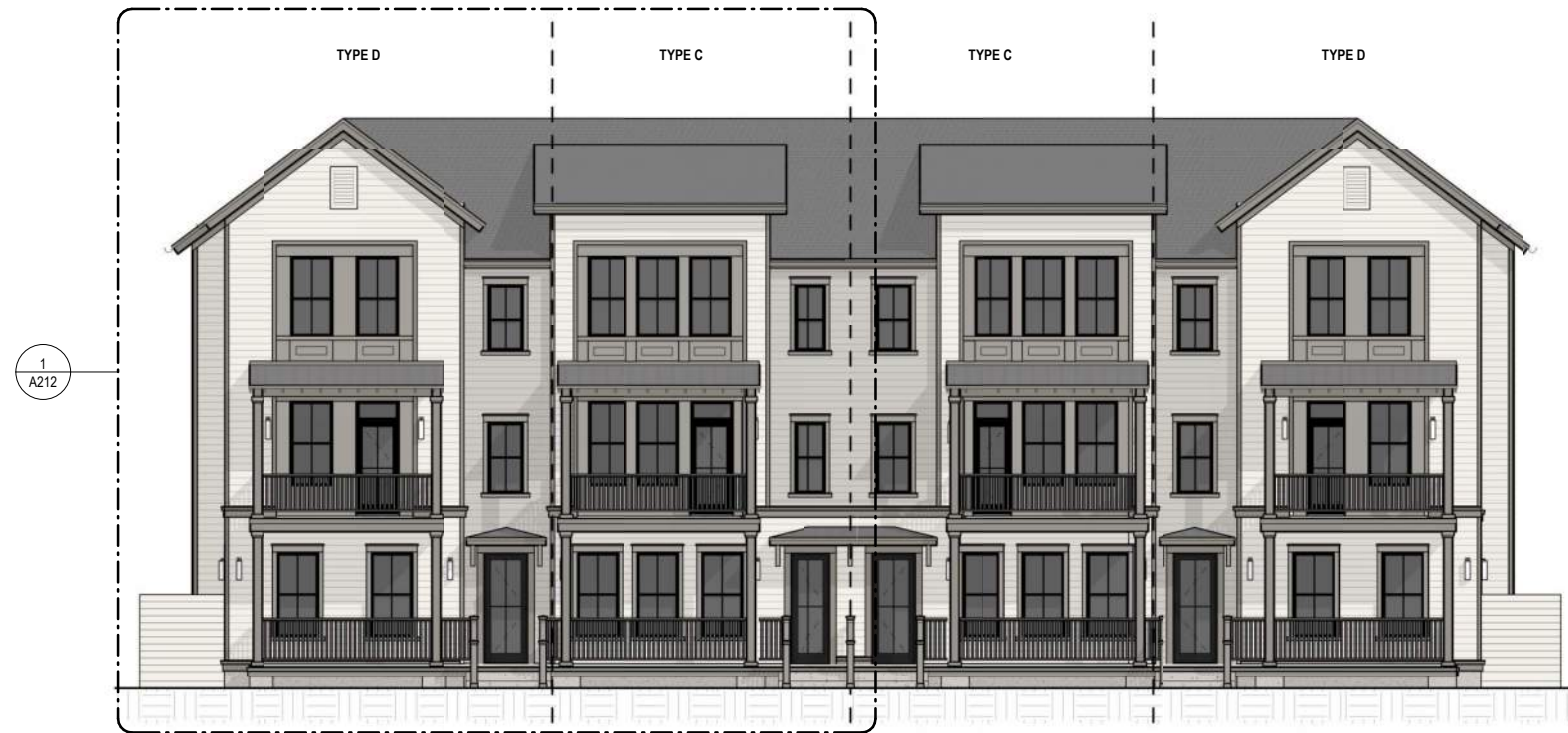
A OVERALL FRONT ELEVATION- BUILDING TYPE 6 A206 1/8" = 1'-0"
